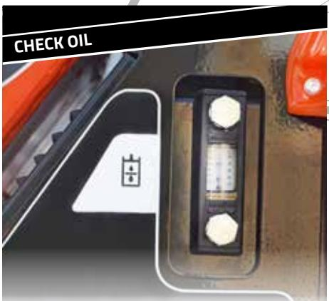
There is a single access point for checking the level, checking the temperature, and filling hydraulic oil.
