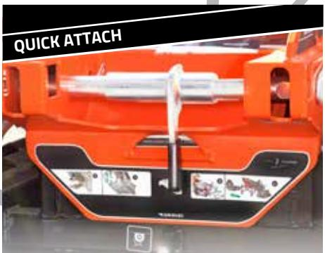
With the Cormidi Quick Attach, you can use a different attachment each time you run the machine (dumper, miniloader, concrete mixer, etc.) Simply attach, check the configuration, and use.
