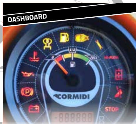
The dashboard provides all your information in one place: tachometer, hour meter, fuel gauge, and alarm light.
